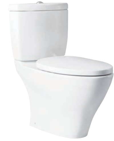
CST940DV Close Coupled Toilet Flush System : Wash Down (6/3L) Bowl Shape : Elongated Rough-in : 305mm 395W x 693D x 793H mm
