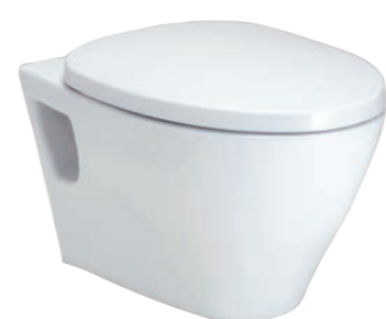
CW941K Wall Hung Toilet Flush System : Wash Down (6/3L) Bowl Shape : Elongated Rough-in : 220mm 360W x 530D x 340H mm
