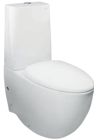
CW811PJ / SW811JP Close Coupled Toilet Flush System : Wash Down (4.5/ 3L) Bowl Shape : Elongated Rough-in : 180mm (P-Trap) 380W x 700D x 845H mm
