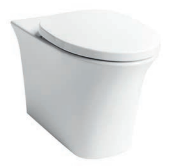
CW193KAU Wall Faced Toilet Flush System : Wash Down (4.5/ 3L) Bowl Shape : Elongated Rough-in : 180mm (P-Trap) 380W x 624D x 390H mm
