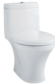
CW630JW / F One Piece Toilet Flush System : Wash Down (4.5/3L) Bowl Shape : Elongated Rough-in : 220mm (S-Trap) 374W x 690D x 705H mm
