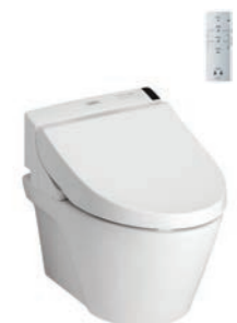
CW822NJ + TCF6531Z Wall Hung Toilet with Washlet Flush System : Siphon (4.5/3L) Bowl Shape : Elongated Rough-in : 220mm (P-Trap)
