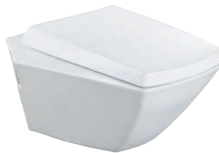
CW682E Wall Hung Toilet Flush System : Wash Down (6/ 3L) Bowl Shape : Elongated Rough-in : 220mm (P-Trap) 452W x 560D x 332H mm
