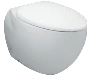
CW813PJ Wall Faced Toilet Flush System : Wash Down (4.5/ 3L) Bowl Shape : Elongated Rough-in : 180mm 380W x 595D x 400H mm
