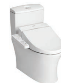
CW920K / SW920K + TCF6631A Close Coupled Toilet with Washlet Flush System : Tornado (4.5/3L) Bowl Shape : Elongated Rough-in : 305mm
