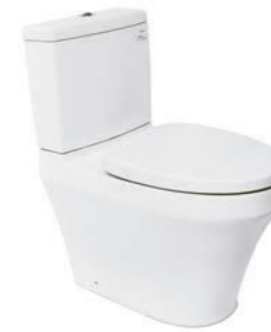
CST945DNN Close Coupled Toilet w/ Seat and Cover Flush System : Siphon (4.8/3L) Bowl Shape : Elongated Rough-in : 305mm 702W x 379D x 806H mm
