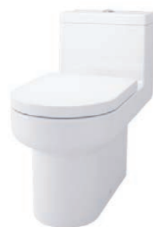
CW895JW/F One Piece Toilet Flush System : Wash Down (4.5/3L) Bowl Shape : Elongated Rough-in : 305mm 360W x 720D x 660H mm
