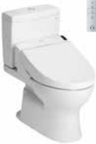
CST320DRV + TCF6531Z Close Coupled Toilet with Washlet Flush System : Wash Down (4.5/3L) Bowl Shape : Elongated Rough-in : 230mm
