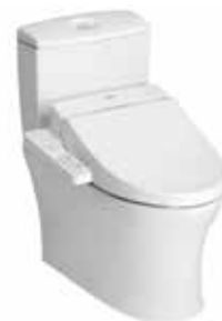
CW920K / SW920K + TCF6631A Close Coupled Toilet with Washlet Flush System : Tornado (4.5/3L) Bowl Shape : Elongated Rough-in : 305mm
